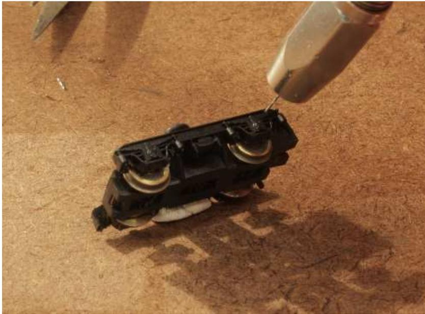
9. Using a 0.4mm drill in a pin chuck, **drill holes for the steps** in the bogies where the bogie frame narrows to a "V". Remember that one bogie has a pair of steps each end and the other only has steps at the outer (coupling) end.
