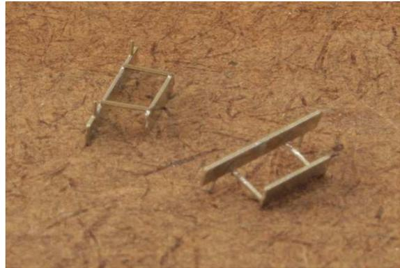
12. **The single steps just need removing from the etch** and the tabs filed off.
