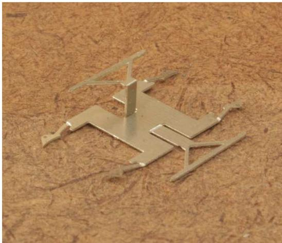
4. Using tweezers, hold the bottom part of the brake below the second fold line, and use your finger or a steel ruler to **fold the top of the brake rigging down 90° so that it is parallel to the floor**. Again do not solder this, but check it is square with the floor.
