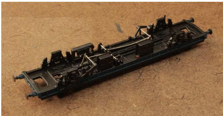
35. When you are happy that everything is straight and true **glue the replacement v hangers to the underframe.** You should be able to lift each v hanger up sufficiently to apply a small dab of glue on the end of a cocktail stick.
