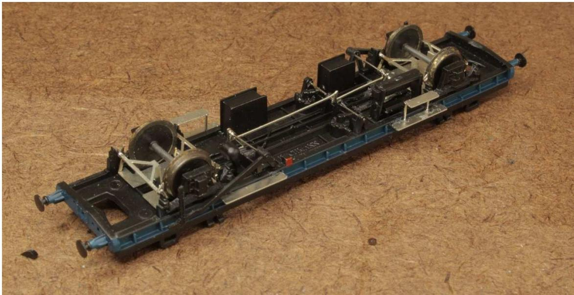
39. Remove the end steps from the etch, bend the bottom step 90 degrees and fix in place on the end of the vehicle. These are placed to the right of the left buffer where they should leave sufficient space for body mounted DG couplings to operate. NEM couplings and bogie-mounted DGs will probably be obstructed by these in which case it is best to omit these steps.
