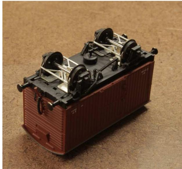
We recommend using a slow-setting glue such as Araldite or Serious glue which gives you time to adjust the alignment of the assembly to ensure it is central with the wagon axleguards. Alternatively you can hold the assembly in place and apply cyanoacrylate to the edges allowing it to penetrate underneath and fix the part in place, but make sure you are 100% happy with the alignment before doing this.
