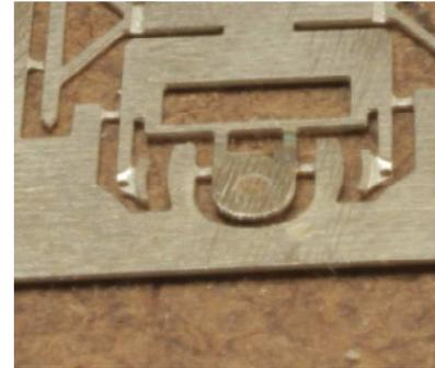
2. In order to obtain sufficient clearance for fitting to the wagon, **the outside faces of the bearings need to be filed down**. Take care when doing this not to weaken the bearing bracket. You can file them flush with the etch (as in the pictures here) but if you leave a millimetre or so it will help with aligning the assemblies on the wagon.
