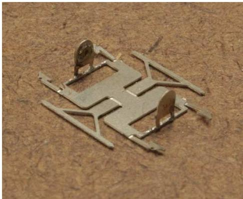
4. Apply a small amount of solder cream to the fold lines next to the bearing brackets. Using a scalpel to start, and a steel rule to finish, **fold the bearing brackets up at 90° to the floor**. At least there is no protruding bearing to get in the way. Check for squareness and **solder in place**.
