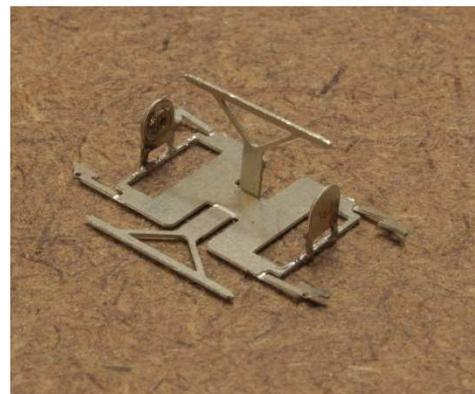
5. The brake rigging is connected to the floor of the etch by a piece of metal that has two fold lines, one on each side. Using a pair of long nosed pliers, hold one piece of brake rigging so that the nose of the pliers is just shy of the fold line, then **bend the entire piece of brake rigging up at 90° to the floor**. Do not solder it as we need some movement here for adjustment later.
